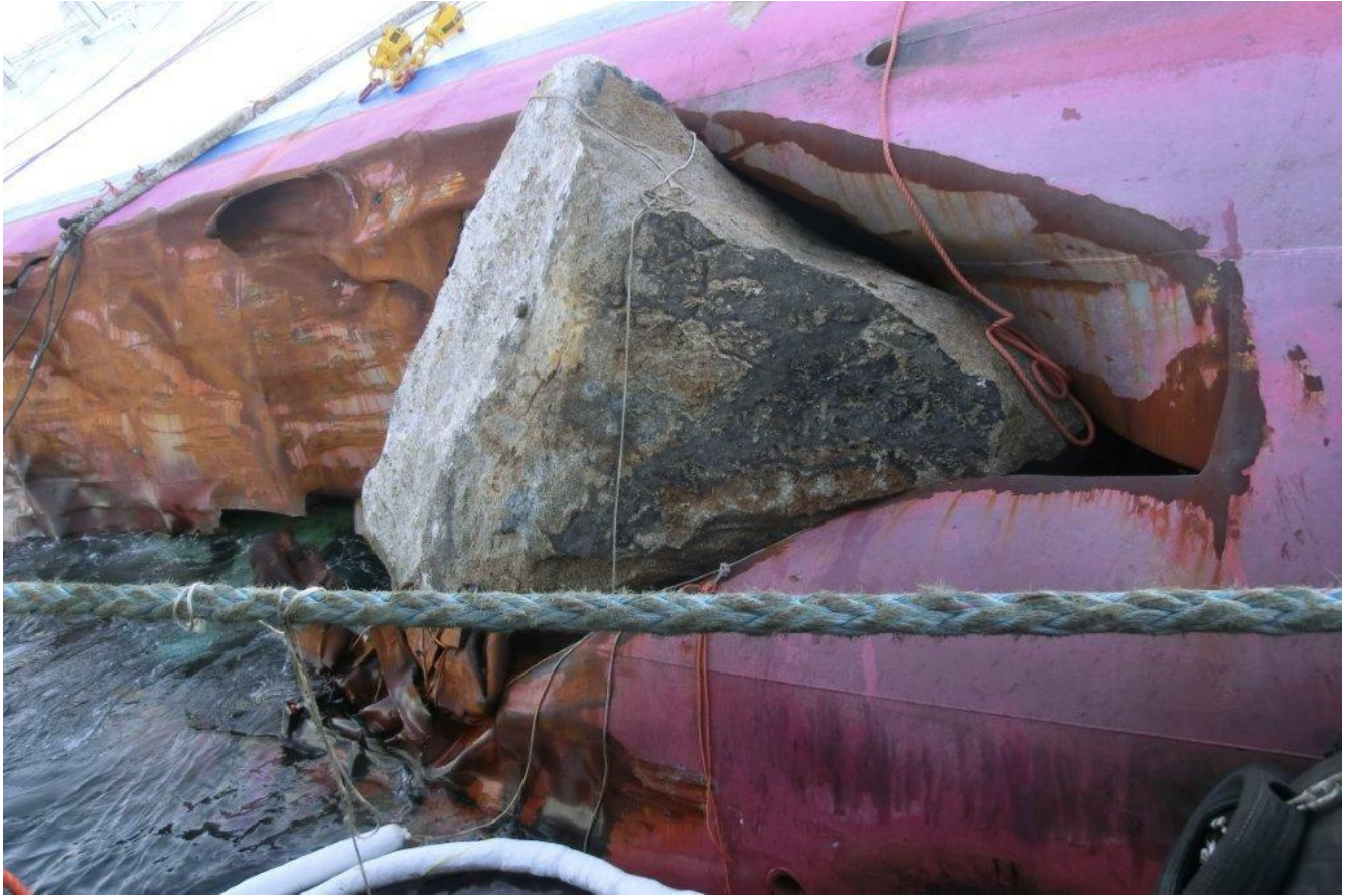
Detached rock in damaged area
